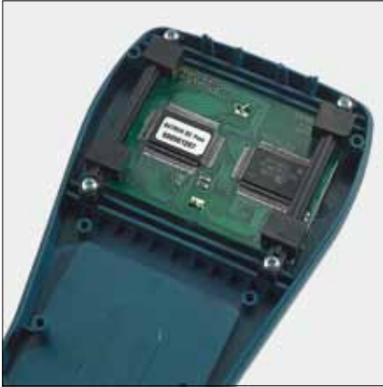
Display fixing set for variable display mounting
