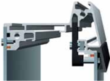
Front panel installation screwed from front
