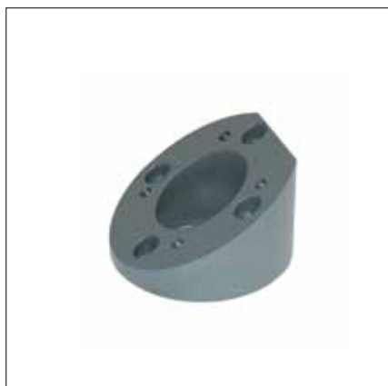
Console flange Aluminium incl. screws and seal, fixed inclination 30°. Screw-mounted between enclosure and coupling.
