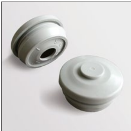
Double membrane connecting plug IP 66, with 2 integrated sealing membranes, interference fit without counter-nut, for wall thicknesses of 1.5 - 4.5 mm
