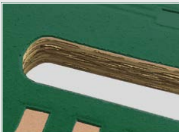
Cutting of mounting holes
