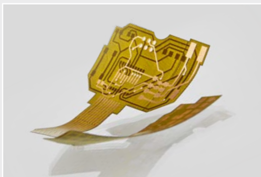
The cutting and structuring of single- and double-sided laminated flexible electronic materials (DuPont Pyralux)
