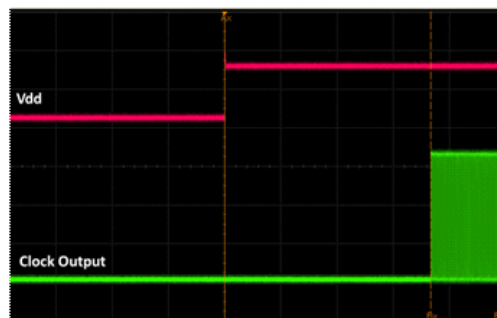
Figure 17. Startup Waveform vs. Vdd
