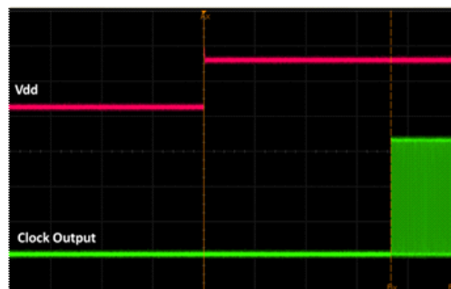
Figure 17. Startup Waveform vs. Vdd
