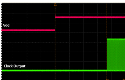
Figure 17. Startup Waveform vs. Vdd
