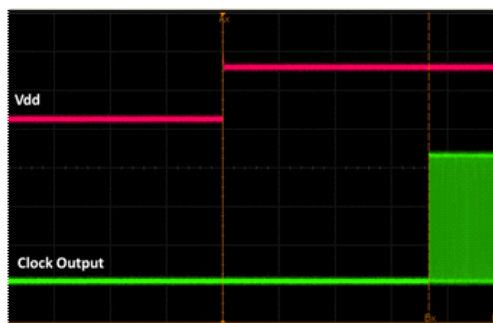
Figure 14. Startup Waveform vs. Vdd
